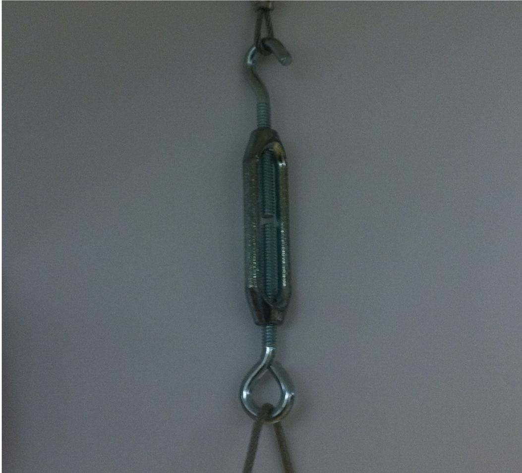
It's best to use an adjustable turnbuckle (as seen above) when the light is hung. The turnbuckle will allow for quick and easy leveling between ends. Turnbuckles and other hardware needed to hang your DIAMOND light can be found at most hardware stores.
